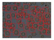
Fig. 6. Example of results given by cascade object detector: Red rectangles represent cells found in the raw image. Cells on the fringes are ignored
