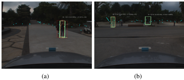
Fig. 4. (a) Detection of two pedestrians with a single bounding box. (b) Detection of a non-pedestrian object.
